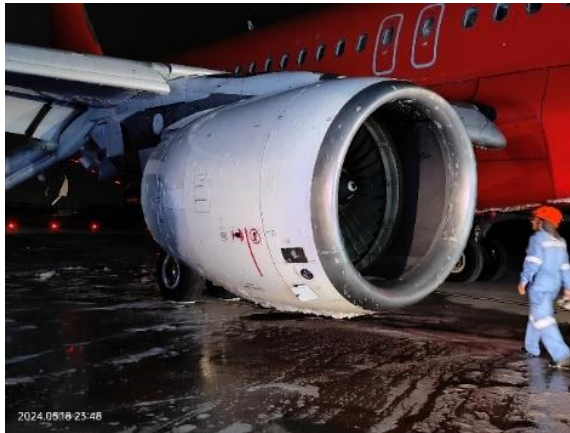
Fig 4 Engine Inlet condition post Fire Extinguishing action by ARFF
