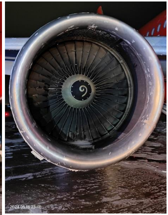
Fig 4 Engine Inlet condition post Fire Extinguishing action by ARFF
