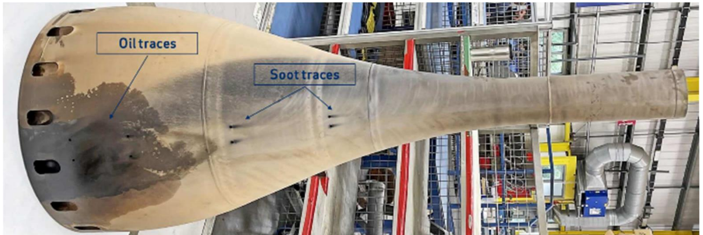
Fig 31 Oil traces and black deposit found on exhaust plug at 06:00 position.
