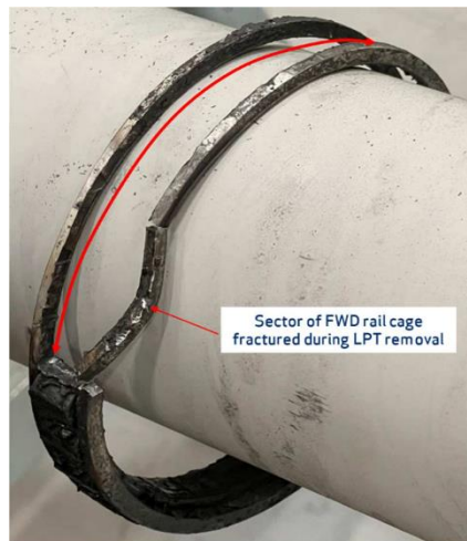
Fig 35 Cage spacers fractured and associated rollers liberated onto a sector of ~180°
